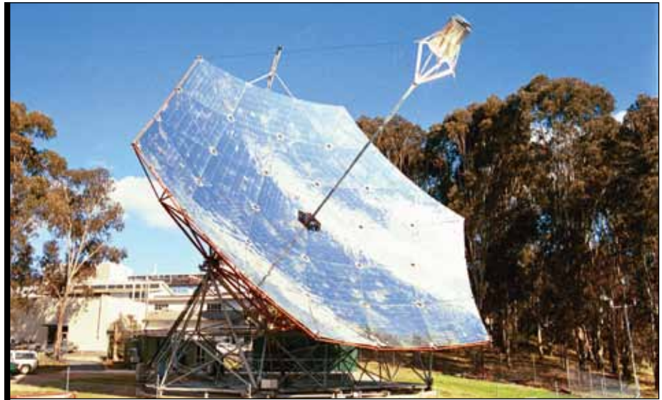
Wizard's 400m 2 Big Dish at ANU and pressure vessels for ammonia-based storage.
