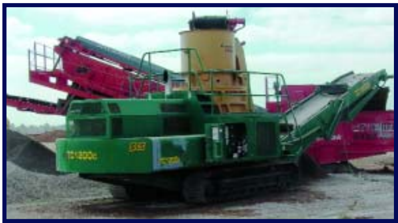
This small-scale, mobile crusher at Tenterfield in Melbourne's northwest brings the advantage of reusing C&D materials on-site.
